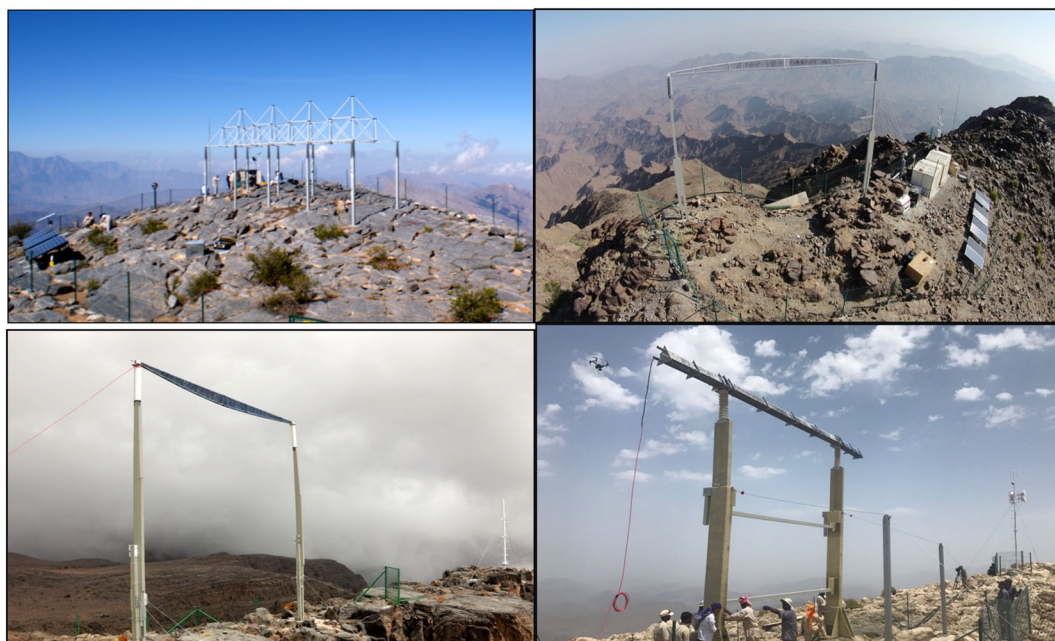
Figure 2. The different ioniser designs used in the Hajar Mountains trial. Top row is the original pyramid design at H2 (left) and fisheye design used at H3 (right). Bottom row is the fisheye design used at H7 (left) and triangle design used at H10. These design modifications aimed to increase the amount of ion flux generated when the device is operating.
